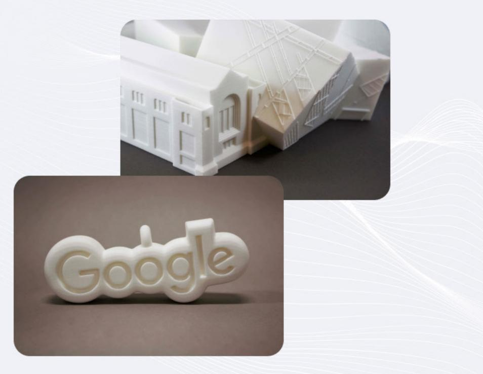
material is joined together one layer at a time to create a three-dimensional object from a computer file. Typically, 3D printing is used by designers and engineers to create one-off or small batch quantities of a valuable part or product.
